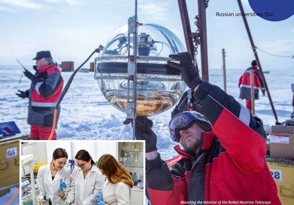
Mounting the detector of the Baikal Neutrino Telescope
